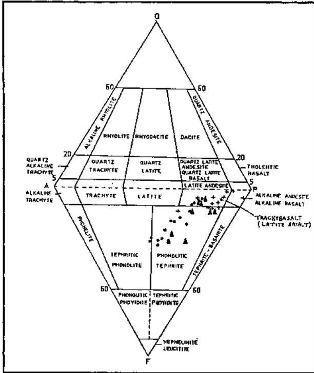
Figure 7. Nomenclature of the basalts according to the Streckeisen (1976) bi-triangular diagram
